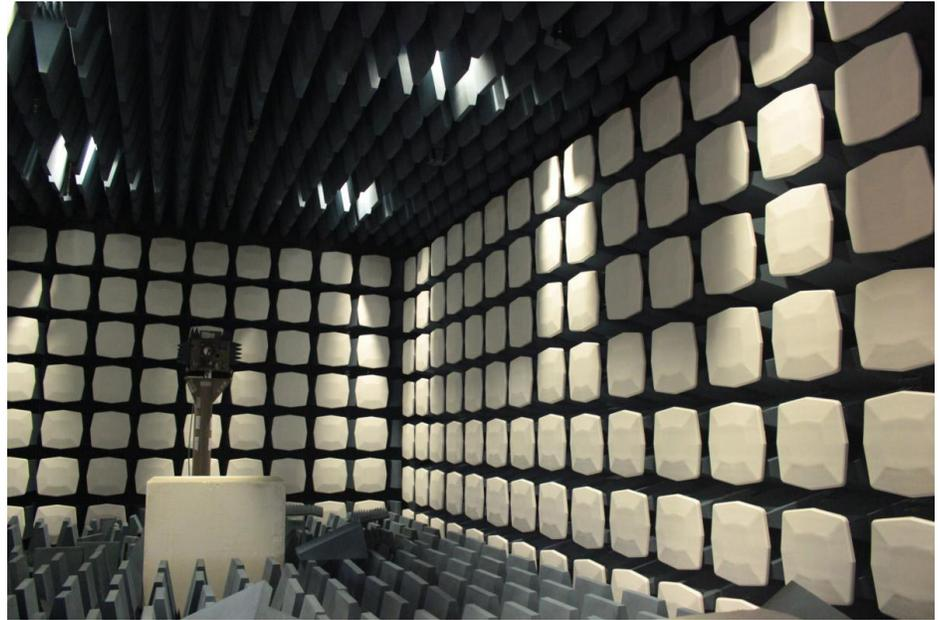
The chamber in the Robust Electromagnetic Field Testing and Simulation Laboratory (REFTAS) determines the directional emissions spectrum from a variety of equipment and systems including unmanned aerial systems and their sensors.
