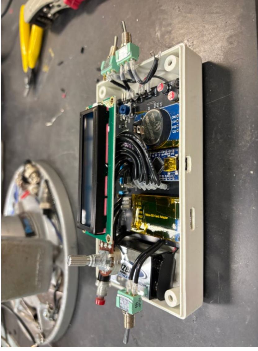
Figure 2. Shows the systems components: printed circuit board (PCB), micro-SD card module, RTC, switches, reset, and a background potentiometer.
