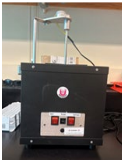
Fig 1. carousel-type UV reactor used for UV photolysis and UV/H 2 O 2 advanced oxidation experiments. UV dose was standardized using ferrioxalate actinometry to ensure consistent treatment conditions.
